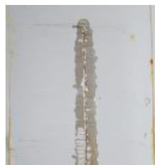
Figure 8: Uses beyond roof coatings; 2K WB epoxy 1.8mil DFT (1032 hours)
