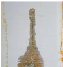
Figure 8: Uses beyond roof coatings; 2K WB epoxy 1.8mil DFT (1032 hours)
