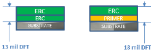
Figure 7: Two coat comparison over G70 Galvanized
