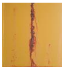
Figure 9: Uses beyond roof coatings; WR Alkyd, 2.2mil DFT (504 hours)
